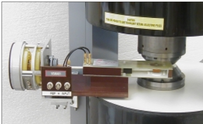
VSM - Vibration and measurement unit
