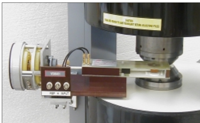
VSM - Vibration and measurement unit
